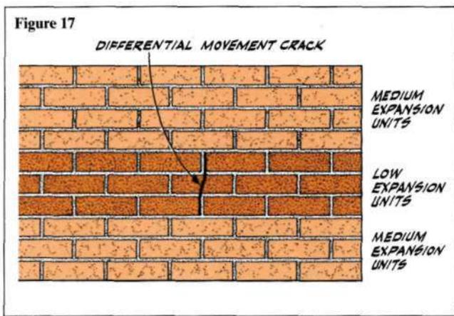
brickwork of another colour. The difference in colour will also result in different thermal movements. The result is that the expanding mass of brickwork puts the string courses into tension and they crack - Fig 17.
