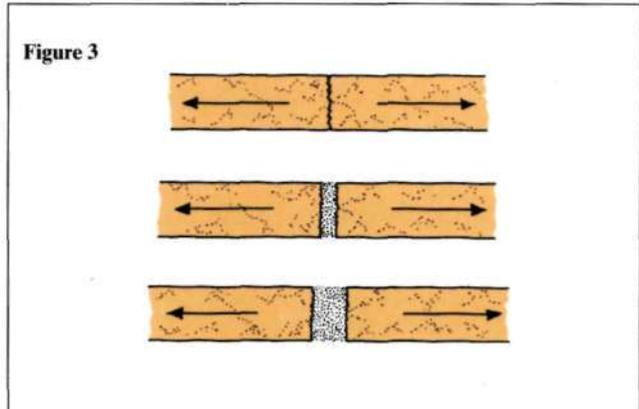
may be more stable and less likely to crack than those allowed to move freely. This may be the preferable design option in some cases. Prestressed concrete is a well known example of the calculated application of this design technique.
